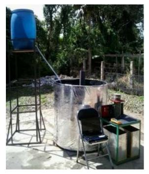
Figure 1: The prototype Salt Gradient Solar Pond (SGSP)
