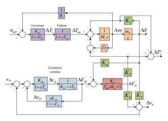
Fig. 2. Single-machne to connected to an infinite bus
