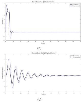
Fig. 7. Simulation results of optimal and uncontrolled control signals in cluster 1, (a) frequency, (b) bus voltage, (c) electrical power
