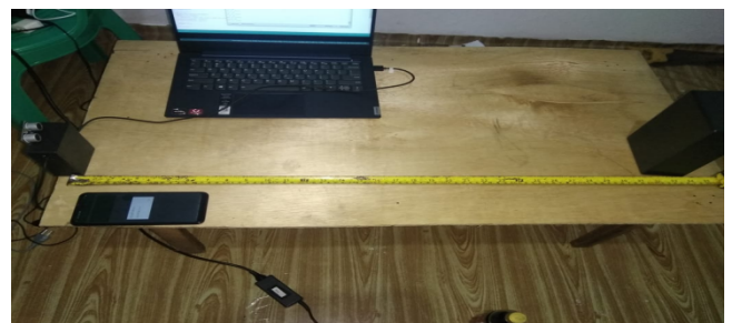
Fig. 5. Ultrasonic Sensor Calibration
