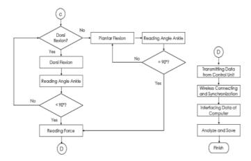
Fig. 12 (b). Flowchart Mechanism System.
