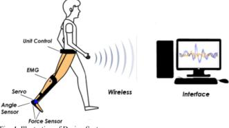
Figure 4 explains that the illustrations shown about this study's design consist of several sensor indicators, namely EMG, angle sensors, and force sensors. The built system to transmit using wireless A networks and display interfaces on the computer in real-time. The explanation as follows.
