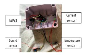
Fig.2. Prototype for the monitoring system of the transformer
