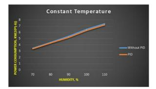
Fig.11. Power Consumption Graph Constant Temperature
