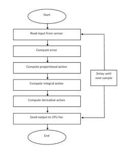
Fig.6. PID Flowchart
