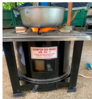
Fig. 12 Firing Test with Biomass Stove
