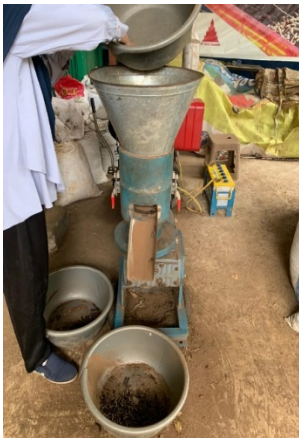
Fig. 10. Calliandra Wood Printing Process with A Pellet Mill Machine
