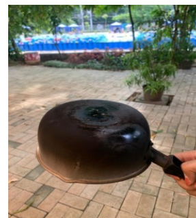
Fig. 13 Soot from Burning Bio-Pellets
