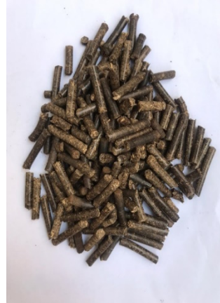
Fig. 11. The Results of Biopellet Molding Calliandra Wood Biopellets With 16% Adhesive
