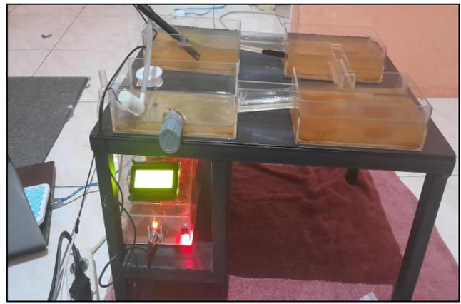
Fig. 11. The Process of Reading the pH Value of Each Pond
