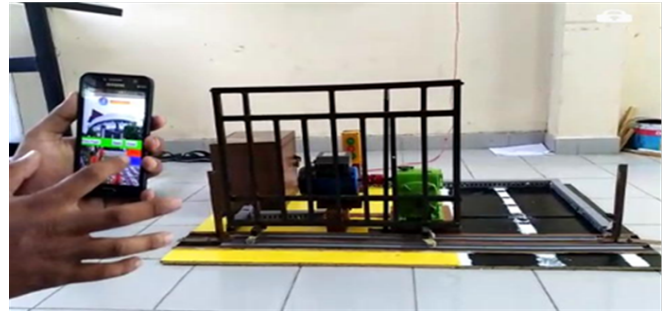
Fig. 10. Sliding gate opener system together with the smartphone as its remote controller.
