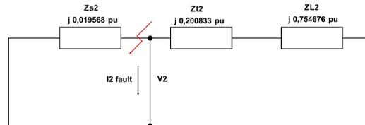
**Figure 3.** Equivalent Impedance Circuit of Negative Sequence at 150 kV
