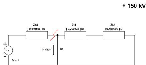
**Figure 2.** Equivalent Impedance Circuit of Positive Sequence at 150 kV
