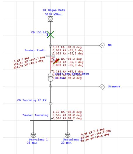
**Figure 5.** Simulation of a Single-Phase to Ground Short Circuit at 150kV
