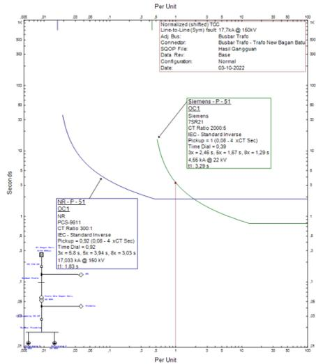
**Figure 7.** 150kV Two-Phase Fault OCR Coordination Curve
