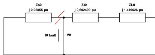
**Figure 4.** Zero Sequence Equivalent Impedance Circuit Fault at 150 kV
