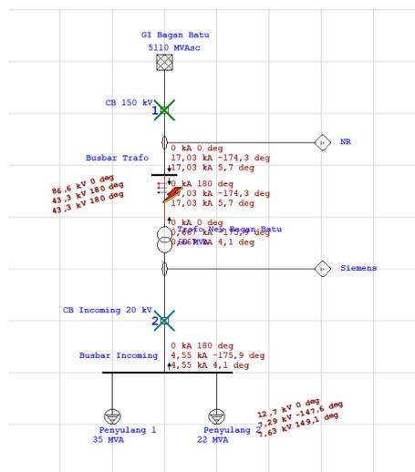
**Figure 6.** Simulation of Two-Phase Short Circuit at 150 kV
