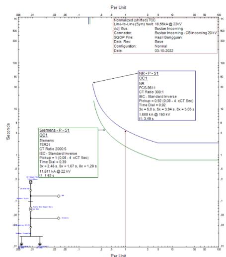
**Figure 10.** 22kV Two-Phase Fault OCR Coordination Curve
