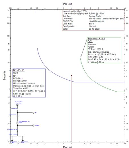
**Figure 8.** 150kV Single Phase to Ground Fault OCR Coordination Curve
