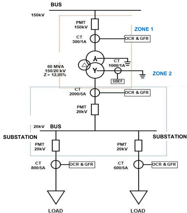
**Figure 1.** OCR & GFR Protection Zone Power Transformer 60 MVA of BB Substation
