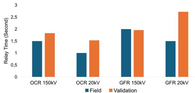
**Figure 11.** Comparison of Relay Working Time
