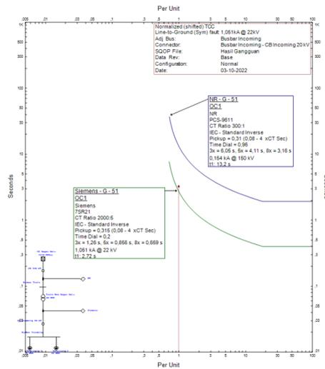
**Figure 9.** GFR Coordination Curve for a Single-Phase Ground Fault 22kV
