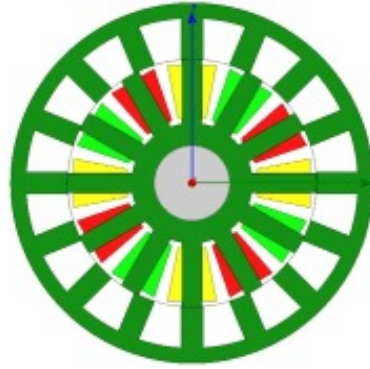
Figure 3. 12/16-pole DOSRG finite element 2D model diagram
