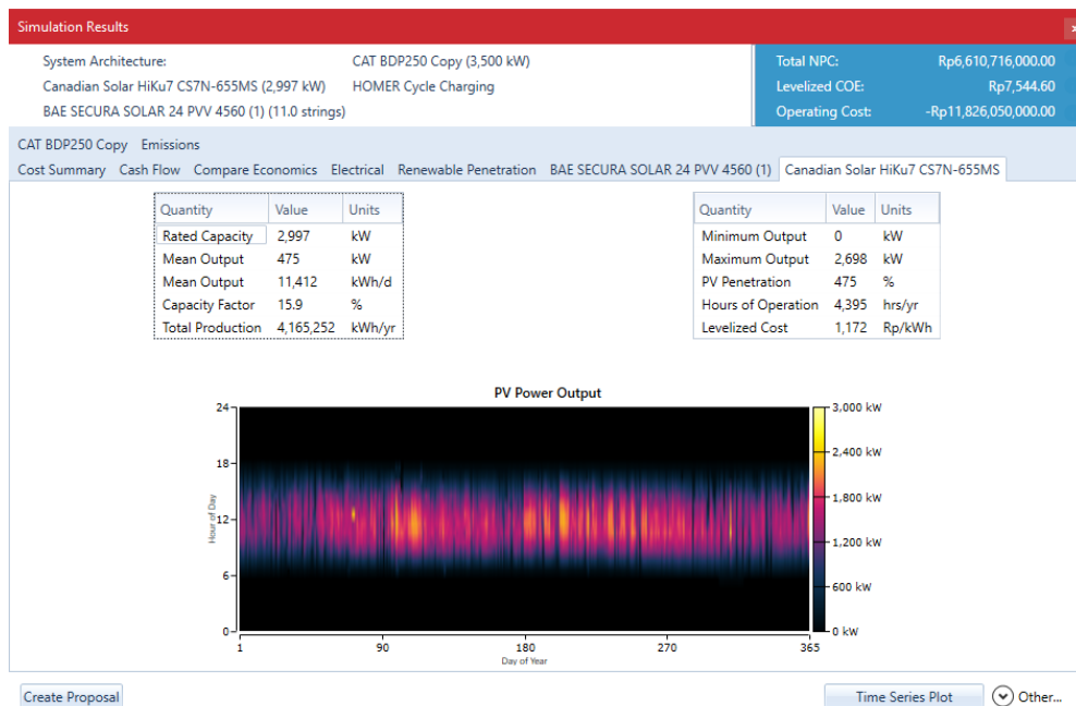
Figure 5. Operational Simulation Results of PV Array CS7N-655MS for The Apartment Building
