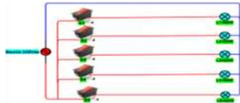
Figure 11. The five input switches On / Off connected to the lamps
