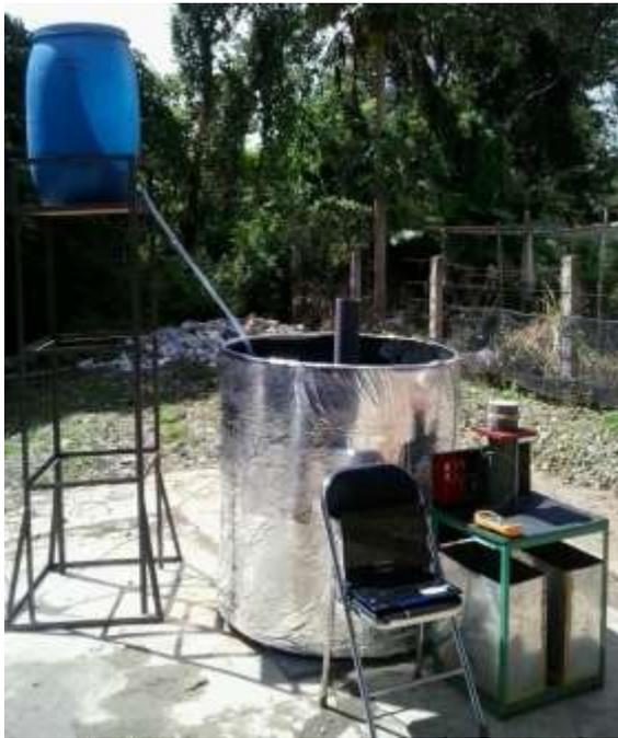
Figure 1: The prototype Salt Gradient Solar Pond (SGSP)
