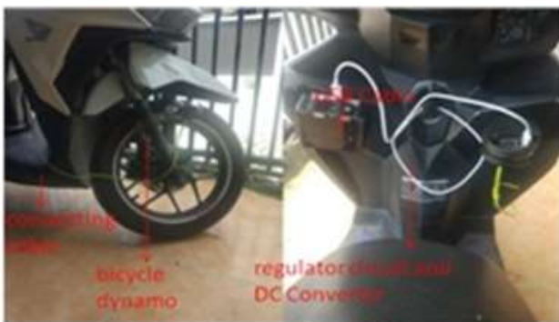
Figure 6: Installation of a circuit on a motorcycle
