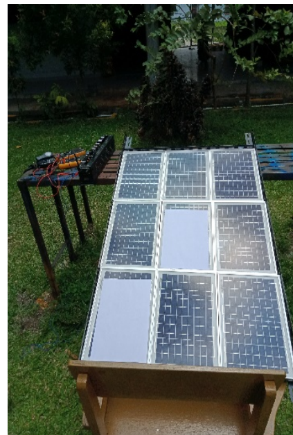
Figure 7. Prototype Photovoltaic Array 9 \times 10 \text{ Wp} With Shading Condition 0 1 1 (22,2%)
