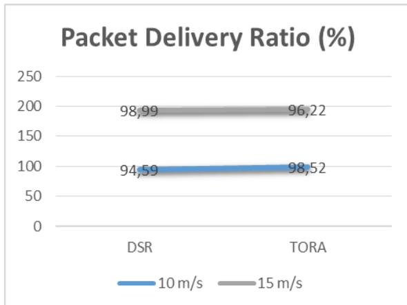
Fig 6. The effect of node speed on PDR in urban scenario
