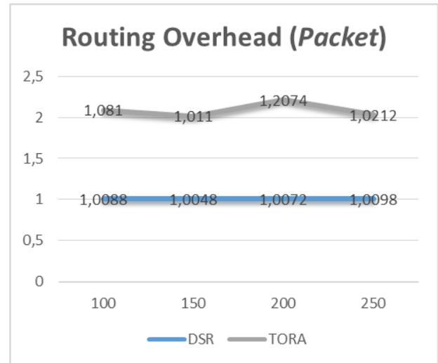
Fig 4. The Effect of number of nodes on RO in urban scenario
