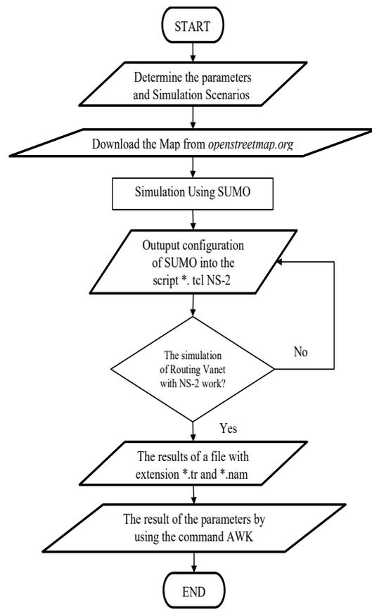
Fig 1. Flowchart design simulation
