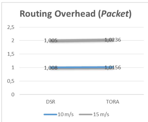
Fig 7. The effect of node speed on RO in urban scenario
