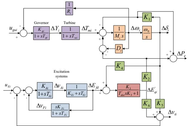
Fig. 2. Single-machine to connected to an infinite bus
