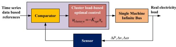
Fig. 1. The proposed load-based optimal control-cluster
