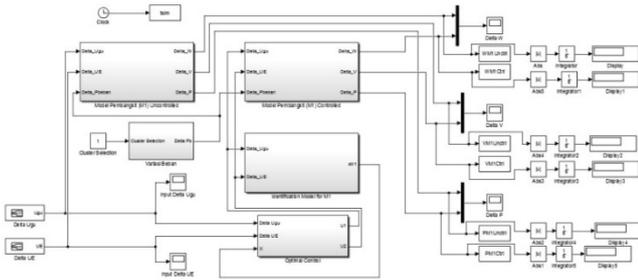
Fig. 5. Representative optimal control model
