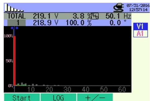
Figure 11: Tests on the system before the filter is installed
