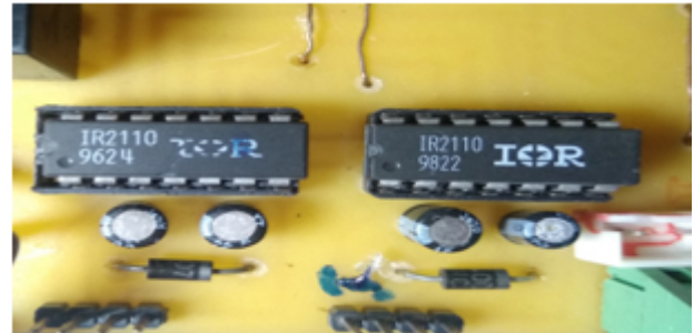
Fig.7 Measurement of SPWM Wave Output IC IR2110 prototype
