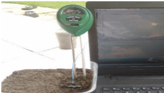
Fig. 13 Validation of YL-69 Soil Moisture Sensor with Soil Meter
