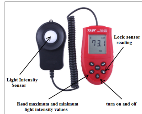
Fig 7. Physical Form and Important Functions of Digital Meter
